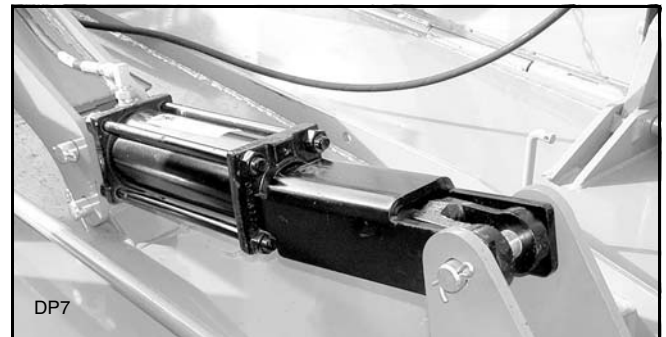
Figure 3. Transport Lock In Transport Position
